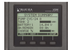
Vessel Systems Monitor
