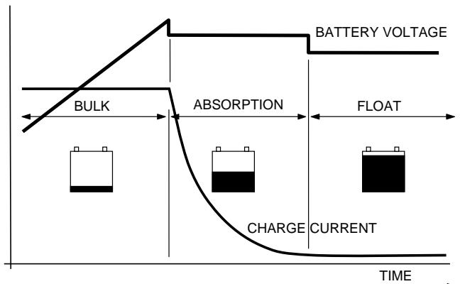
Three-stage charge curve: Stage A: BULK, for quick charging from 0 to 80%, Stage B: ABSORPTION, the battery is charged from 80 to 100%. Stage C: FLOAT, battery is maintained in fully charged state.
