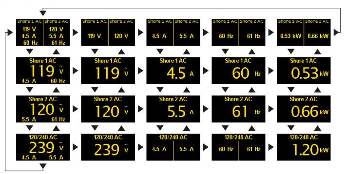
Press the **Menu** button to bring up a shortcut menu to for additional summary screens as well as to access the Setup menus. Press the **UP** ↑ and **DOWN** ↓ arrow buttons to move the cursor over the options and press the **Select** button to see a selected display. To return to the previous display, press the **Back** button.
