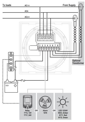
For more information regarding Current Transformer placement in 120/240 Volt AC Systems, refer to the following article: https://www.bluesea.com/support/articles/AC\_Circuits/86/Current\_Flow\_in\_120\_240\_Volt\_AC\_Systems
