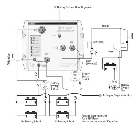
NOTE: This diagram has all of the elements of the ProlsoCharge models. Additional alternators or charging inputs will follow the same basic configurations.
