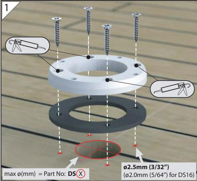
Choose a rubber seal with a central hole  $\varnothing$  that is the closest fit to the  $\varnothing$  of your cable.
