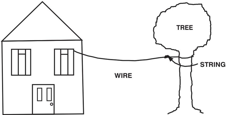
*Tie the end of the antenna wire to a piece of string which in turn is tied to a tall object.*
