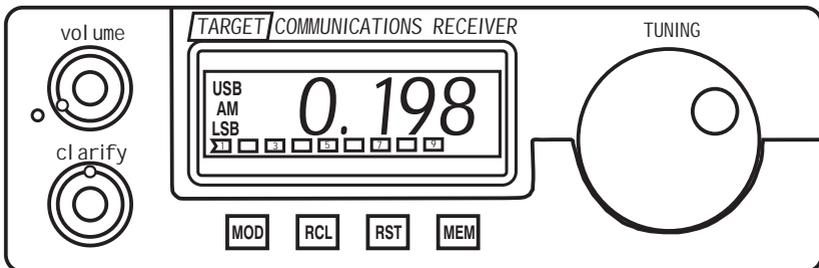
The **TARGET HF3** receiver covers the entire spectrum from 30 kHz to 30 MHz.
