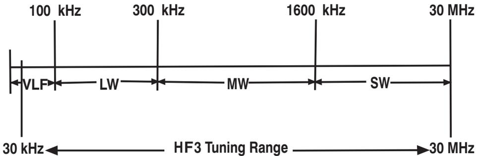
The **HF3** covers all of these bands in one continuous sweep with steps of 1 kHz. Numbers to the left of the decimal point are in MHz whilst those to the right are in kHz.
